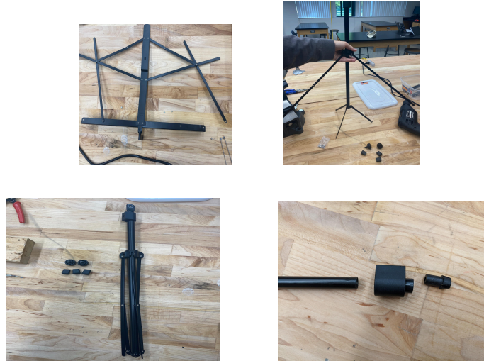
Figure 5. (Some images of the disassembly process, including the removal of rivets from the frame and the detachment of the upper and lower shaft)
